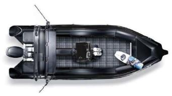
Arctic-Bort specialists have developed a new prototype of a boat made of ultra-strong material with rigid cylinders each with a diameter of 500 mm. The main forms of planing contours are made in the form of Triklin, which makes it possible to instantly exit the vessel onto the glider, without significant motor loads.
