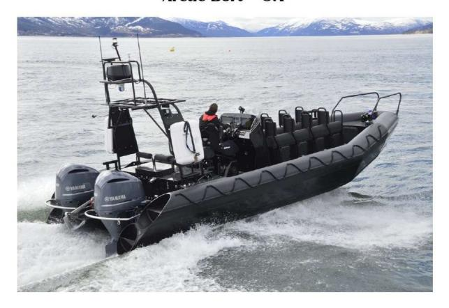
Arctic-Bort specialists have developed a new prototype of a boat made of ultra-strong material with rigid double cylinders each with a diameter of 500 mm. The main forms of planing contours are made in the form of Triklin, which makes it possible to instantly exit the vessel onto the glider, without significant motor loads.
