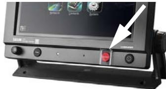
During this time the button light flashes and the buzzer sounds. After 3 seconds the red light goes steady on and the buzzer is silent. The display shows that the message is being sent.
