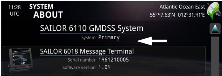
If you have an Alarm Panel in the system, the primary and duplicated systems will appear in the Alarm Panel as Inm-C 1 and Inm-C 2 respectively.
