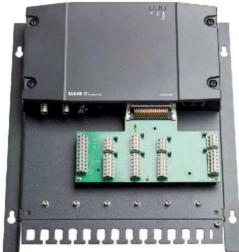
Figure 6: SAILOR 6283 AIS Connection Box and Wall Tray
