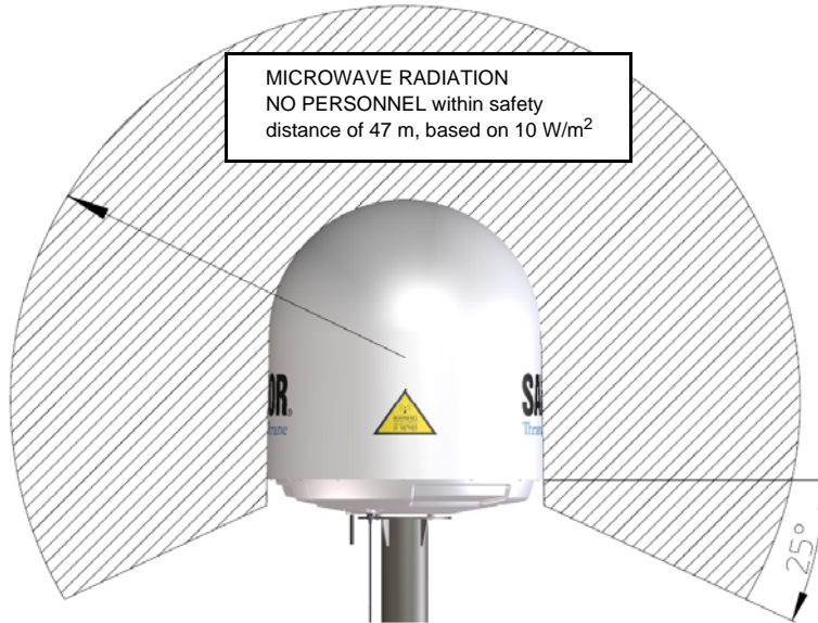
Figure 3-4: SAILOR 900: Radiation hazard, safety distance 47 m
