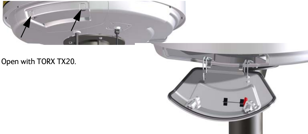
Figure 3-19: Opening the service hatch
