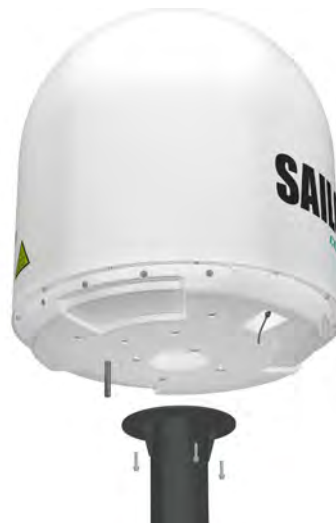
Figure 3-17: Mounting the ADU on the mast flange
