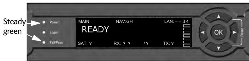
Figure 5-1: ACU display after first power on (example with LAN ports 1 and 4 used)
