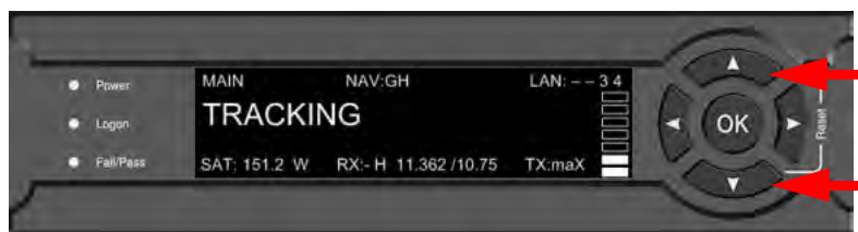
Figure 6-38: Reset the system
