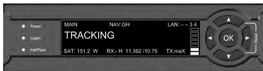
Figure 4-2: ACU: LEDs, display and keypad (detailed)
