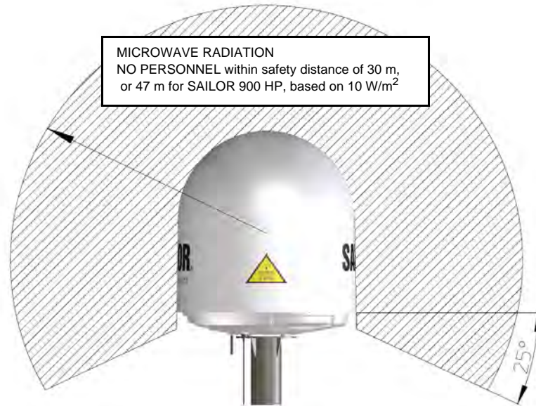
Figure 3-4: Radiation hazard, safety distance 30 m or 47 m (SAILOR 900 VSAT Ku High Power)
