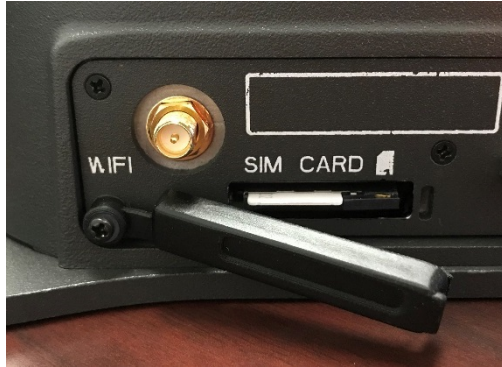
Figure 3-3 SIM Card with Cover Opened
