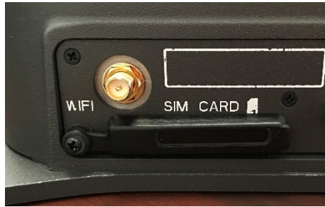
Figure 3-5 Secure the SIM Card Cover
