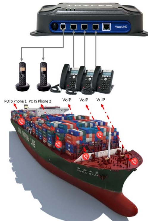
Figure 2-2 Local Communications via PBX Functionality
