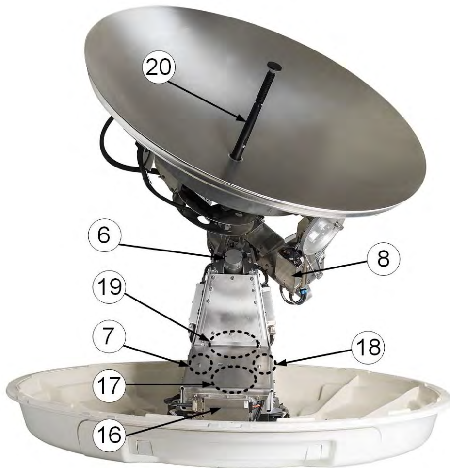
Figure 2-5: Above Deck Unit modules 2/2
