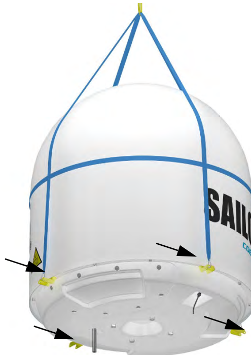
Figure 3-16: ADU installation, webbed sling attached to the 4 lifting brackets
