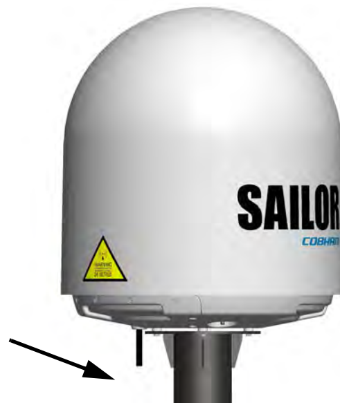
Figure 3-13: Drain pipe with free space
