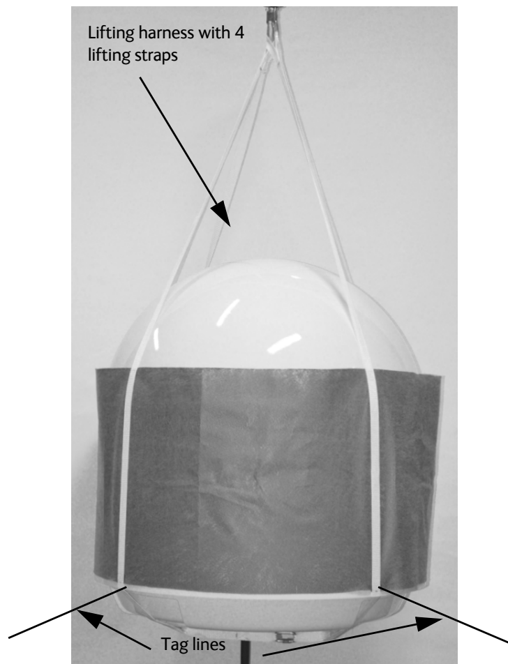
Figure 3-18: Use of the lifting harness and tag lines for safe hoisting
