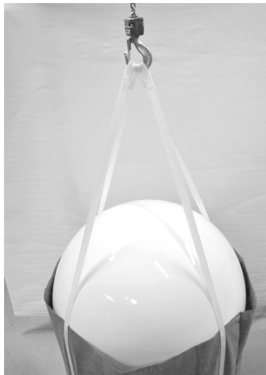
Figure 3-19: ADU installation, 4 lifting straps on crane hook
