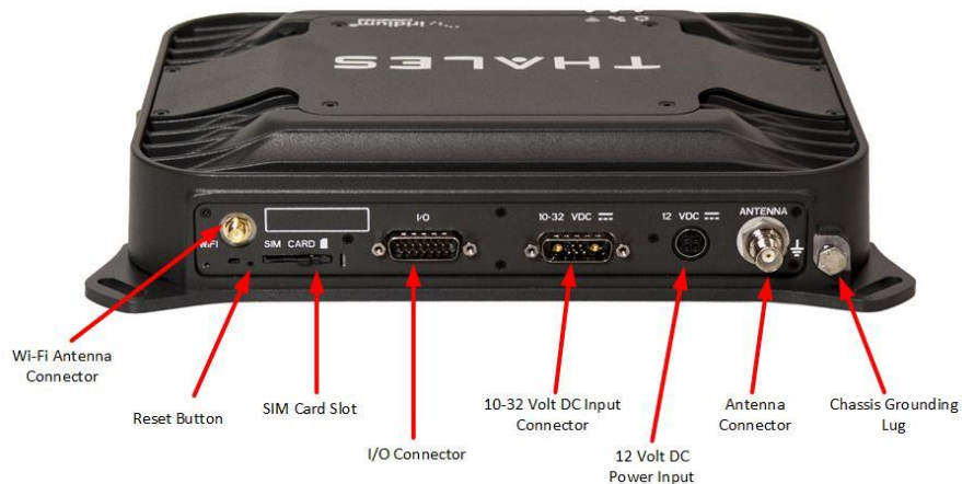
Figure 1-5 Below Deck Unit (BDU) Back Panel Detail
