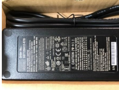
Figure 2-15 AC/DC Power Supply
